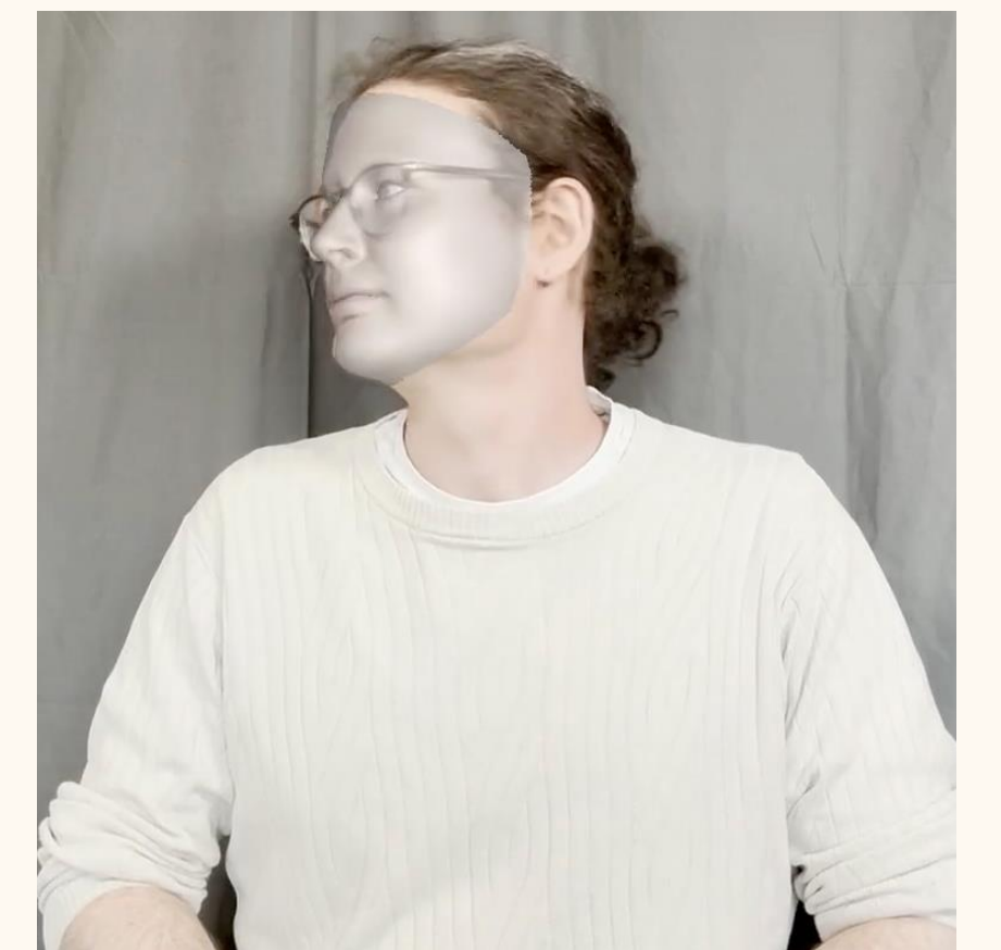
Head pose and face tracking with 3DDFA_v2
