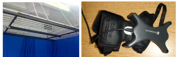
Figure 10: Close-up views of the hand-mounted sensor used in the motion capture sub-corpus data collection.
