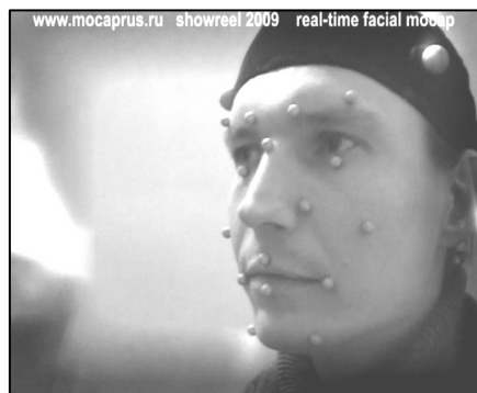
Figure 4: Demonstrator with glued on the face reflectors
