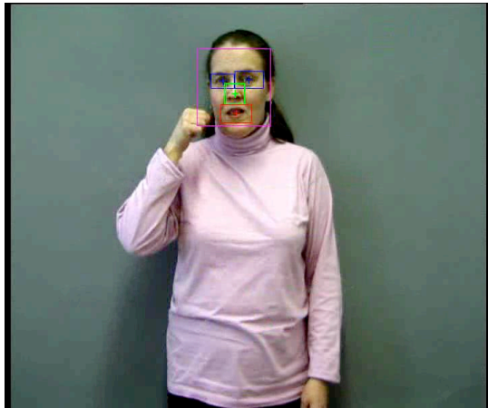
Figure 3: An example of face detection from a recorded sign language video. The detected eyes, nose, and mouth are also shown with separate bounding boxes.
