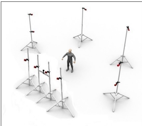
Figure 3: Setup of the ten-camera optical motion capture as well as the HD video camera in our studio
