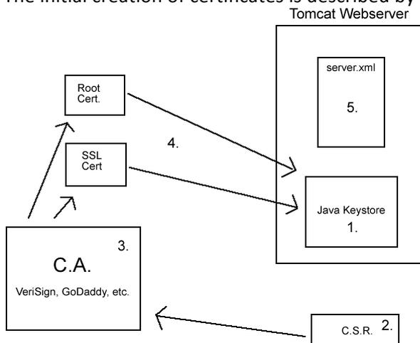
Figure 7: SSL Processing in Tomcat
